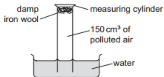
The apparatus is left for one week, during which the oxygen reacts with the iron wool. After this time, the volume of gas in the measuring cylinder is  $122\text{cm}^3$ .
