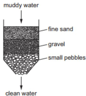
Which process for purifying the muddy water is shown?
