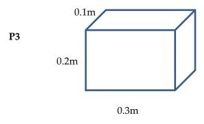
A rectangular wooden block has a mass of 15kg and dimensions of 0.1 m by 0.2 m by 0.3 m. On Earth 1kg weighs 10N.
