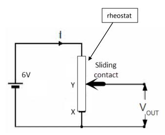
As the sliding contact is moved along the wire, the output voltage (V<sub>out</sub>) changes in proportion to the length of the coil wire between the two points of contact ie points X and Y.
