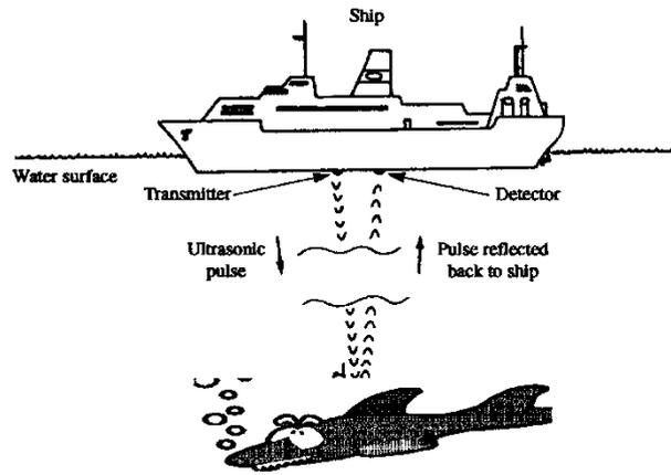
(c) The time taken to receive the echo is 0.2s after transmission. Calculate how deep the ship has to lower its fishing nets to catch the top of the shoal.
