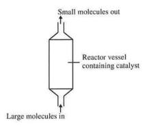
Cracking involves a thermal decomposition reaction.
